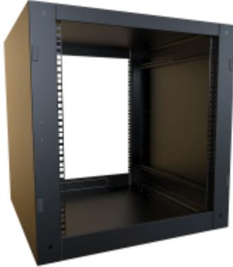
Ideal for AV or IT/Server applications, the RCSC Rack Cabinet features a stacking design that allows for up to three (3) cabinets\* to be stacked atop each other. This Rack Cabinet is fully loaded and includes two (2) pairs of infinitely adjustable sliding EIA square-hole rails, punch-outs for cable entry and/or fan cooling and comes in a variety of sizes and depths.
