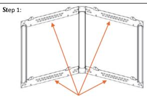
Remove mounting frame from wall mount cabinet. Turn mounting frame so that the eight beveled tabs face up. Position the mounting frame in corner and use the obround (oblong) holes to secure the mounting frame to the corner.
