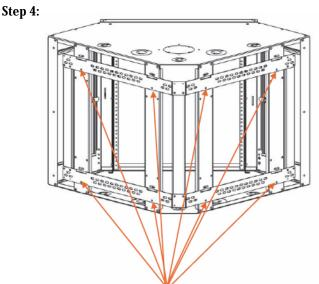
(Optional) Install wall mounting screws (not provided) for additional security in these eight (8) locations to secure the cabinet to the mounting frame.
