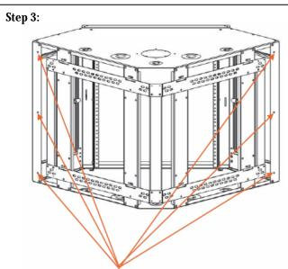
Install screws from the inside of the cabinet(not provided) in these six (6) locations BEFORE installing any equipment in the cabinet.
