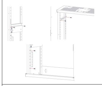
Step 4: Use a screwdriver to remove button head screws. Move the rail to the desired location. Use screw driver to fasten rail into place.
