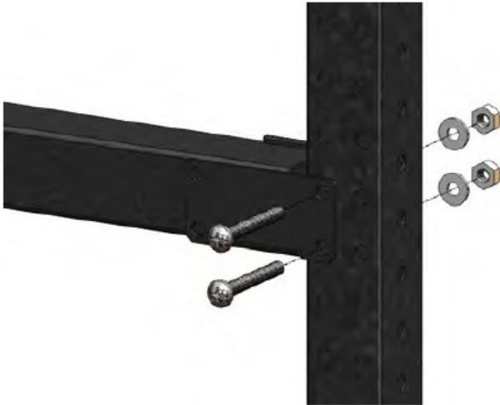
Slide both mounting brackets on either end of the Accessory Bar. Install the bolts through the mounting bracket into the desired position on upright. Install the flat washers and nuts from the backside.
