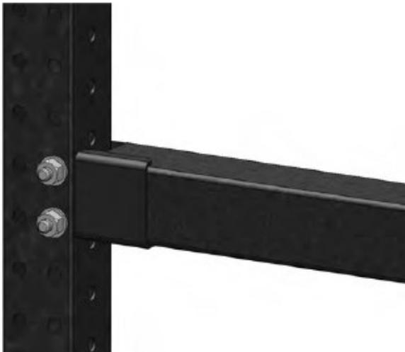
Use the screwdriver and wrench to secure hardware in place.
