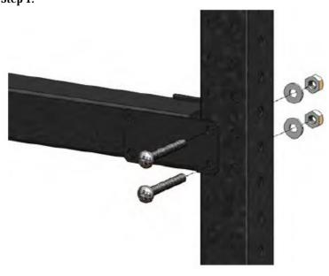
Slide both mounting brackets on either end of the Accessory Bar. Install the bolts through the mounting bracket into the desired position on upright. Install the flat washers and nuts from the backside.
